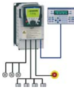
↑ Fig. 8 Section of a conveyor system driven by an ATV71 with an integrated controller card
