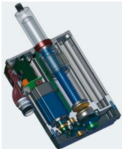
↑ Fig. 41 High performance electric screwjack
