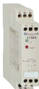
↑ Fig. 15 Electronic device (LT3 - Telemecanique) to be associated with three thermistor probes, for controlling a motor stop when is overheating
