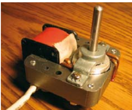
↑ Fig. 10 Single phase short circuit phase-shift rings
