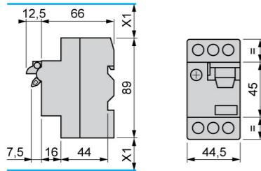
X1: Electrical clearance = 40 mm for  $U_e < 690$  V
