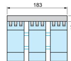
**Note:** Leave a space of 9 mm between 2 circuit-breakers: either an empty space or side-mounting add-on contact blocks.
