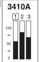
The and buttons may be used to display the currents on the three phases. If the operator no longer uses the buttons for a few seconds, the bargraph returns to the display of the most heavily loaded phase.
