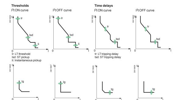
tg: ground-fault tripping delay
