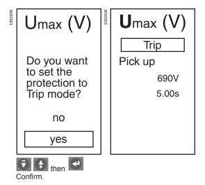
For protection tripped by a maximum value, the dropout threshold is always less than or equal to the pickup threshold.
