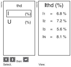
Measure the total harmonic distortion (thd) of the voltage (with respect to rms value)
