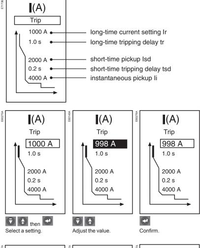
When all the settings have been adjusted, quit the screen by pressing one of the menu-access buttons. This saves the new values.
