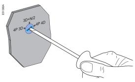
Caution! With the 4P 3D setting, the current in the neutral must not exceed the rated current of the circuit breaker.
