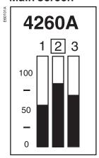
As long as no functions are activated, Micrologic H control units display in real time the current on the most heavily loaded phase.
