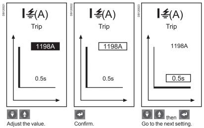
When all the settings have been adjusted, quit the screen by pressing one of the menu-access buttons. This saves the new values.
