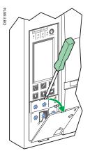
3. completely remove the long-time rating plug screw
