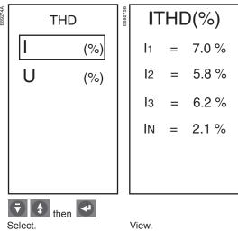
Measure the total harmonic distortion (THD) of the voltage (with respect to fundamental)
