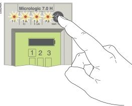
Press and hold down the test button on the control unit to check the LEDs and the battery. The battery information is displayed if the control unit is equipped with an external power supply or if the circuit breaker is ON.
