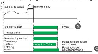
■ Contact operating diagram for the other protection functions
