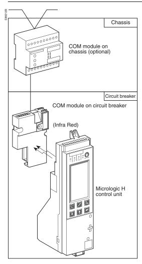
**Communication options**Digipact and ModBus are the indispensable elements when integrating Micrologic H in the Digivision and SMS Powerlogic installation-management systems which communicate via the BatiBus and ModBus protocols.
