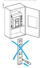
When the door is closed, the crank can be inserted.
