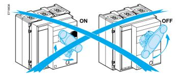
**Note:** the rotary handle can equipped for locking by both padlocks and keylocks.
