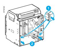
To put the rails back in, press the release tabs and push the rails in.
