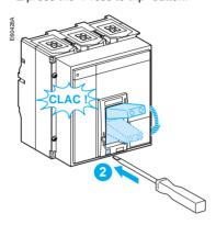
■ push the toggle down to reset the device, then back up close it again.
