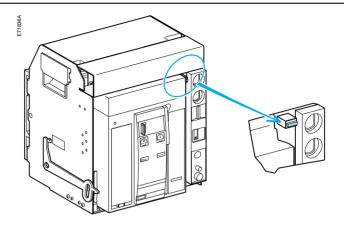
When the door is open, the crank cannot be inserted.
