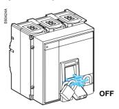
Locking the toggle in the ON or OFF position using one to three padlocks (shackle diameter 5 to 8 mm)  $\,$
