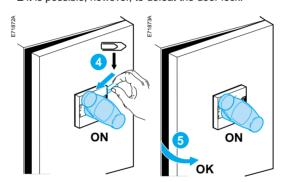
$\blacksquare$  the door-lock function may be permanently disabled by removing the lock.
