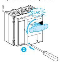
■ turn the handle to reset the device, then back to close it again.
