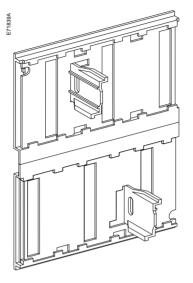
Top shutter locked. Bottom shutter not locked.
