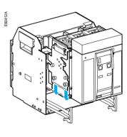
If you cannot insert the device in the chassis, check that the mismatch protection on the chassis corresponds to that on the device.
