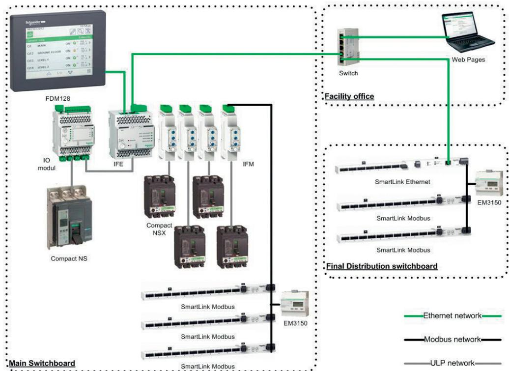
In this application Enerlin'X FDM128, Enerlin'X IFE and Acti9 Smartlink must be connected to the same Ethernet network. So Enerlin'X FDM 128 a must be manually configured to be compliant with both connected products Enerlin'X IFE and Acti9 Smartlink Ethernet, with their respective default IP addresses.
