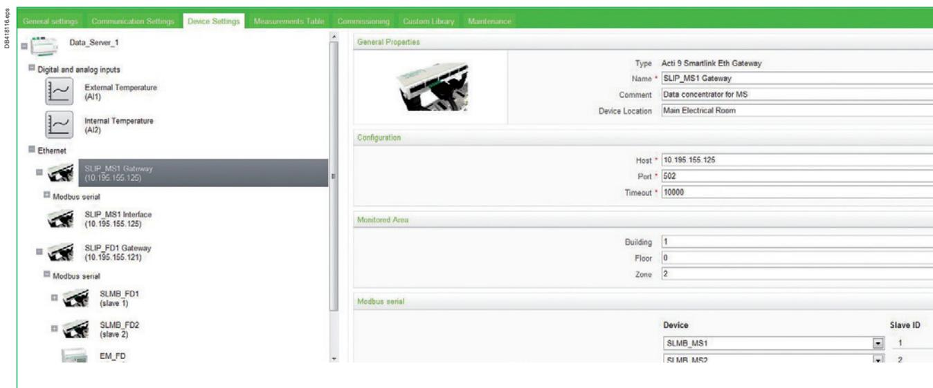
Acti9 channel association needs to be completed for each Acti9 Smartlink in the Com'X 200. Fill in as much information as possible in the Com'X 200. This may include information like localization and description to be ensured analysis of energy data is done correctly.
