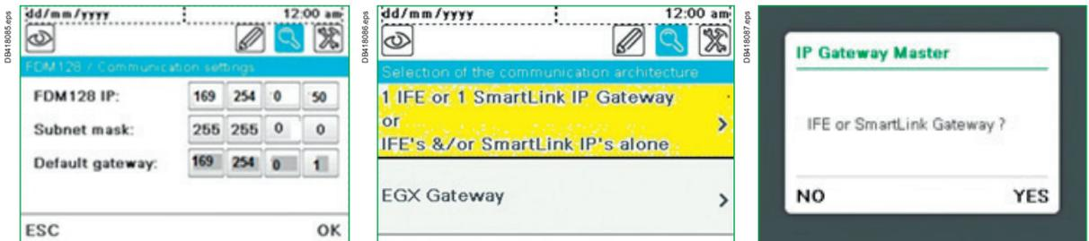
Enter the IP address of Enerlin'X IFE, launch the Modbus auto discovery and select the 6 devices selected for the main switchboard.
