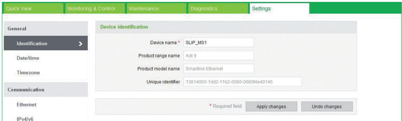
In this section, two Acti9 Smartlink Ethernet devices are used. To reduce the risk of errors, it is recommended to connect them one by one on the Ethernet LAN.
