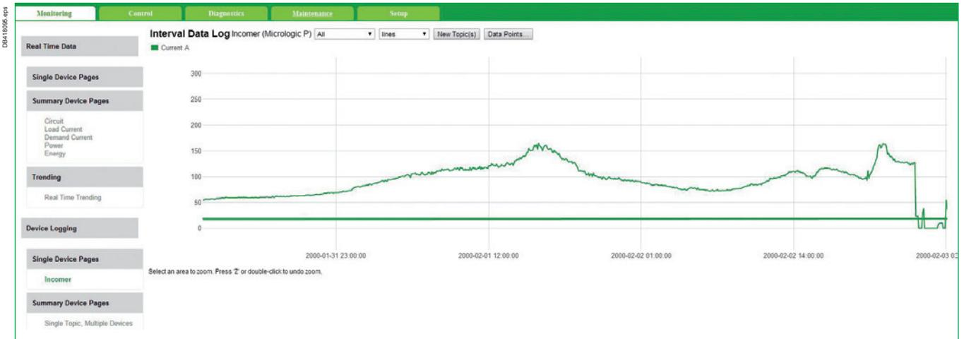
For example, Enerlin'X IFE can store up to three months of data in memory with a 5 sec logging interval. The collected data points may be exported using FTP to a CSV formatted file.
