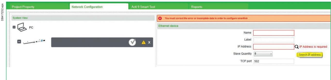
Acti9 Smartlink devices, Ethernet version, will appear automatically when configured correctly. Identify the master and each slave that must be declared:
