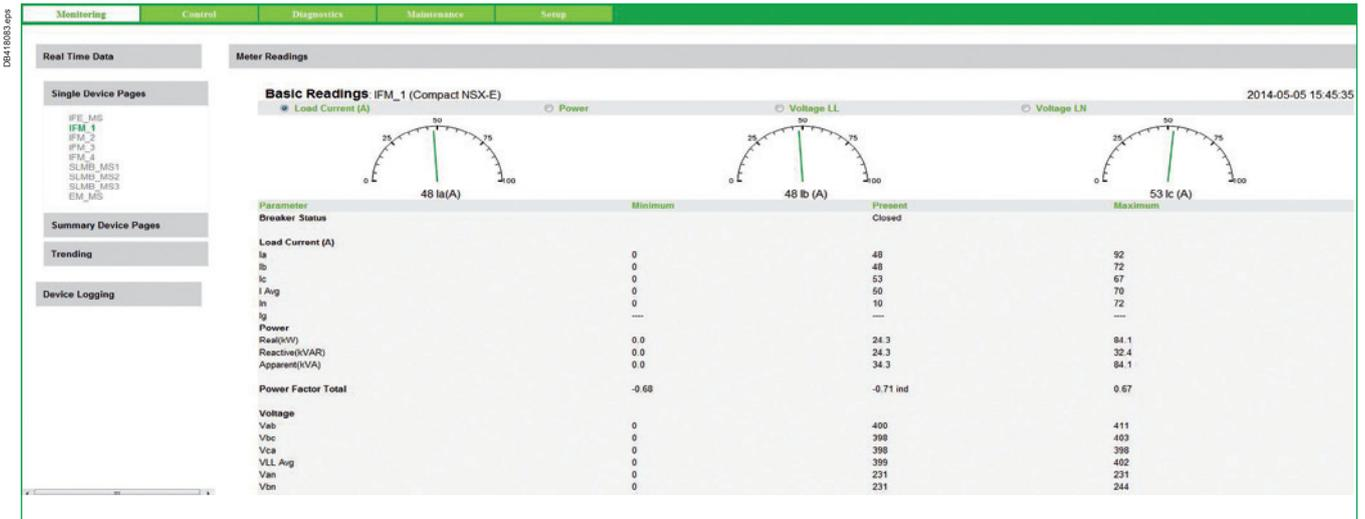
From Acti9 Smartlink web pages, monitoring real time data are displayed and control channels are available for remote controlled devices:
