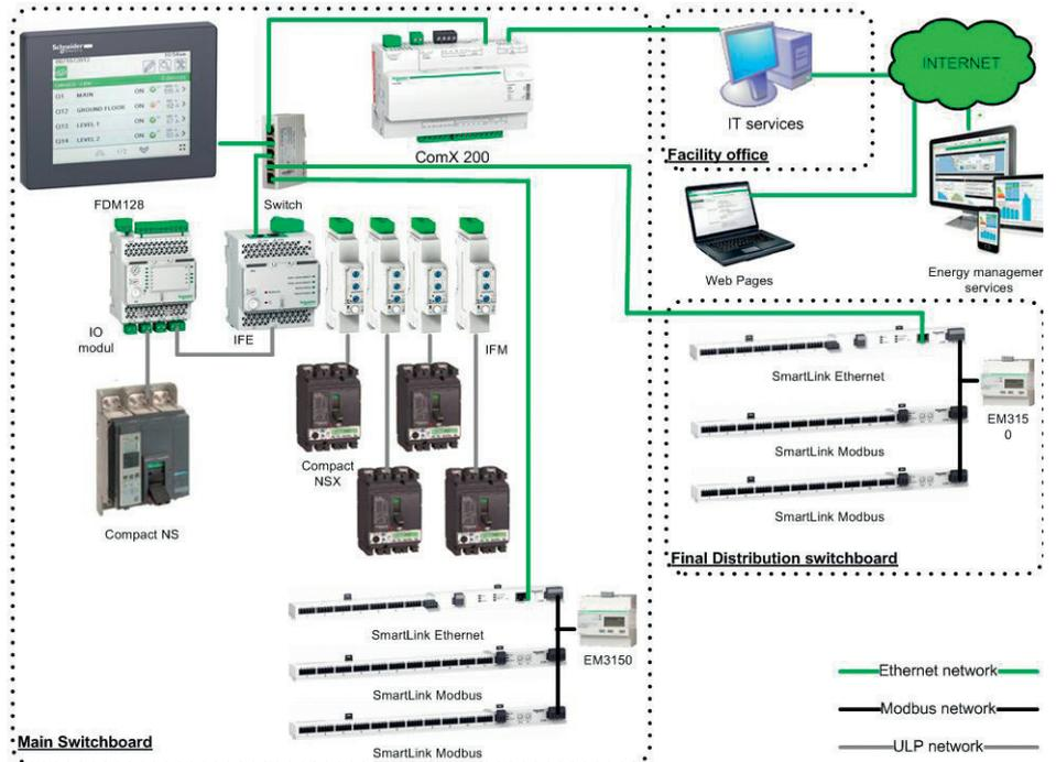
In this application, an IT service manages the addressing rules to connect the Smart Panels to the building network infrastructure. IP addresses are distributed in fixed mode by a DHCP server. This is done to prevent changing Enerlin'X IFE and Acti9Smartlink IP addresses that are manually configured in FDM128 and Com'X 200.
