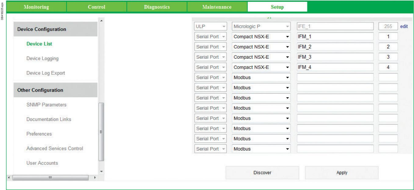
Enerlin'X IFE provides an auto discovery feature of connected Modbus slave devices.
