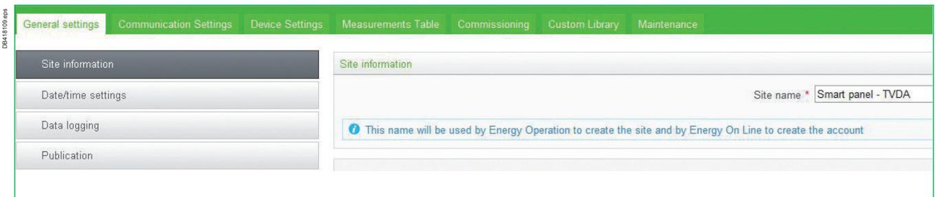
Each WAGES data set can be stored using its own data logging frequency (e.g. electrical values having faster variations than temperature). The image below shows data publication settings in the Schneider Electric on-line energy management service “Energy Operation”. These settings are provided by Schneider-Electric and must be shared with the building IT services to allow data exchange with the cloud.
