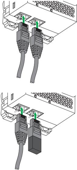
Check the connection between Enerlin'X IFE, I/O interface and circuit breaker using the “ULP test button”. Press the test button on IFE and visually check that IFE, I/O interface and associated Micrologic trip unit flash simultaneously (ON: 1000 ms/OFF: 1000 ms):
