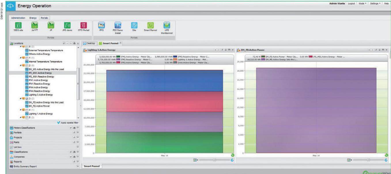
WAGES data points received from Com'X 200 are stored here and can be selected to create an energy dashboard. Site to site comparison is also supported. To enable this feature, contact your Schneider Electric support.
