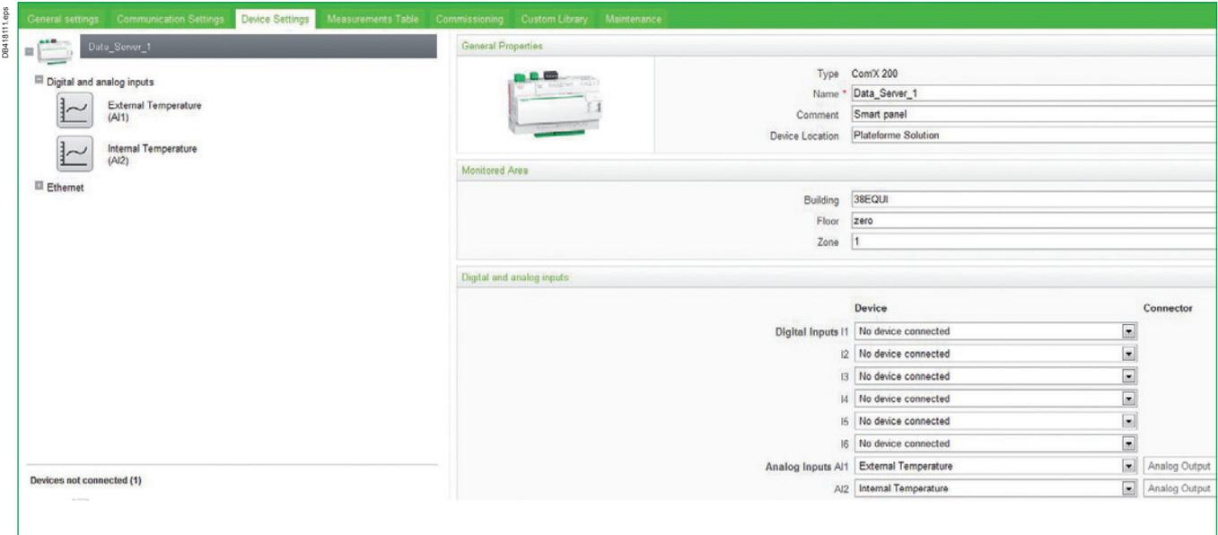
Configure the Com'X 200 energy server to collect data from IFE\_MS, SLIP\_MS1 and SLIP\_FD1 over Ethernet network:
