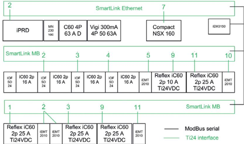
Acti9 Smartlink devices transfer data from Acti9 final distribution devices to a monitoring system via the digital network. Prefabricated cables (Ti24 interface) allow an easy connection of Acti9 devices:
