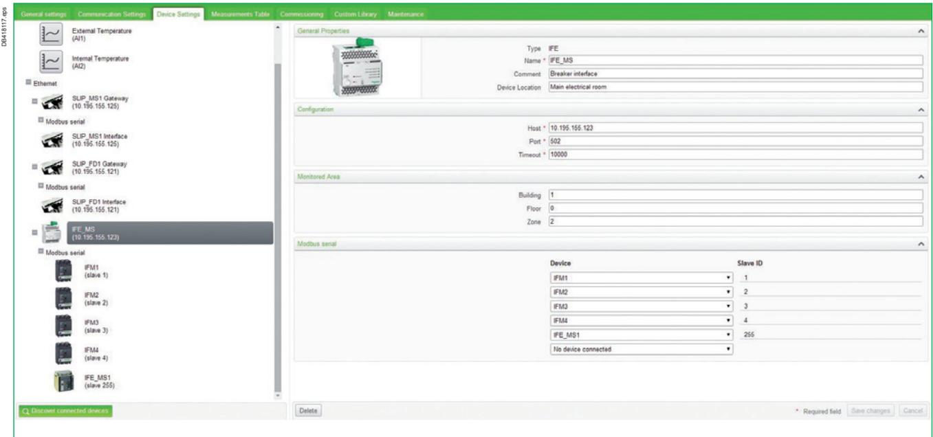
Add one Enerlin'X IFE on the Ethernet network of the Com'X 200 and launch auto discovery via the Modbus serial line (manual configuration is also possible). Enter the correct names of the detected circuit breaker.
