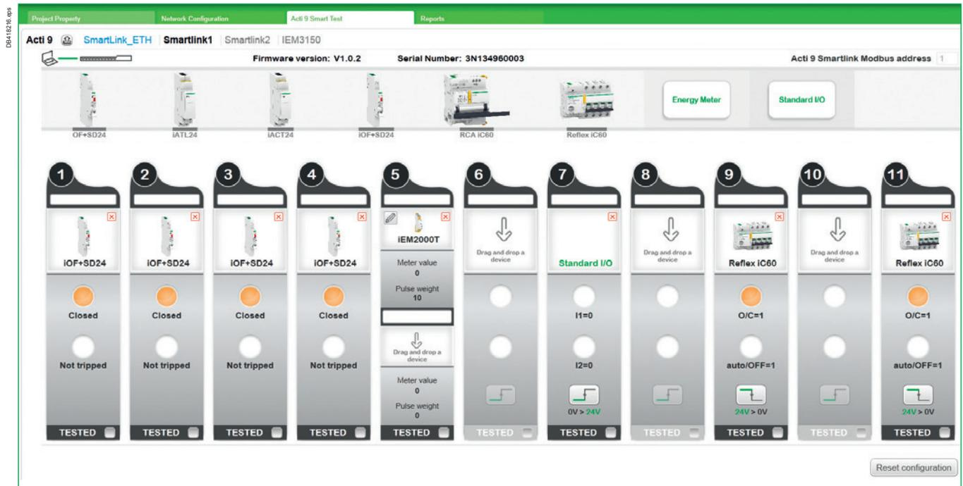
Both communication and functional aspects of each Acti9 Smartlink can be tested with the software. An automatically generated report can be used to supplement contractual documentation in a project.
